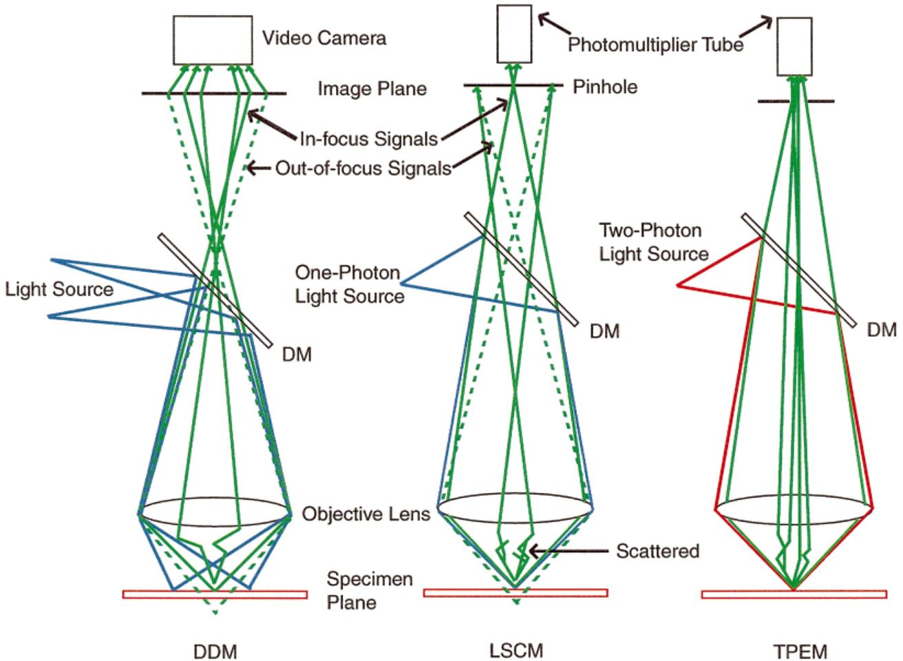
Fig. 3. Illustration of light illumination and detectors configuration used in one- and two-photon imaging systems. DM, dichroic mirror.
