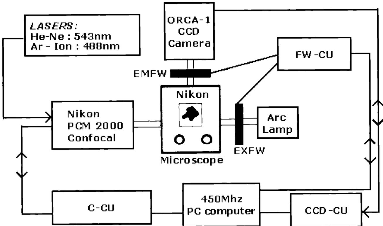
Fig. 1. Schematic illustration of LSCM and DDM. EMFW, emission filter wheel; FW-CU, filter wheel controller; EXFW, excitation filter wheel; CCD-CU, CCD camera control unit; C-CU, confocal control unit.
