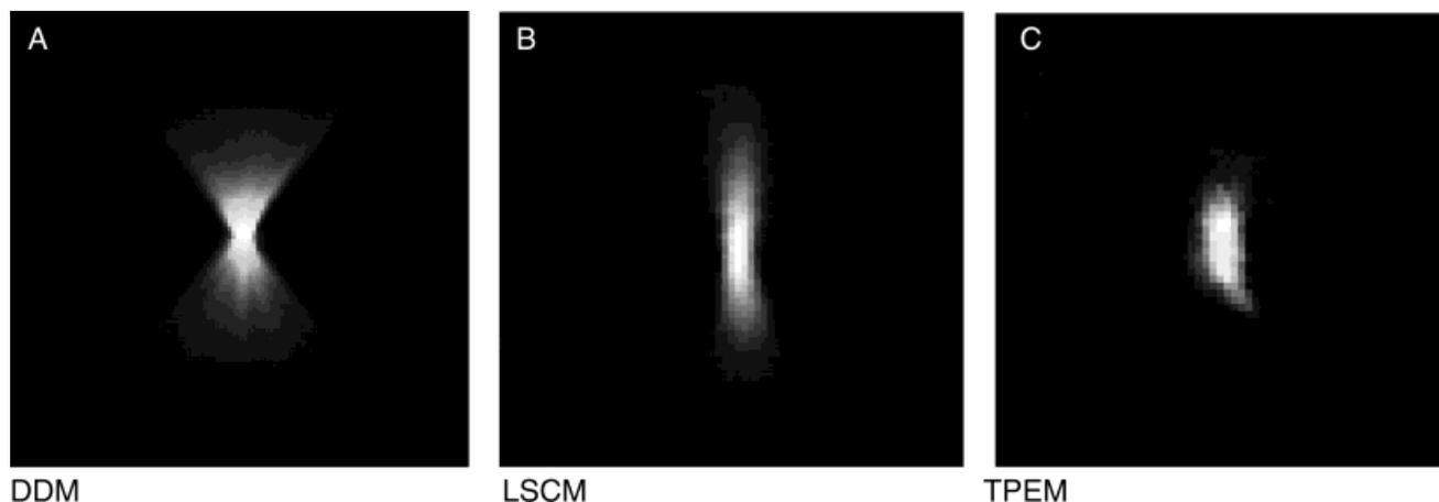
Fig. 2. Three-dimensional reconstruction of point spread function (PSF) of one-micron bead (20X water immersion Plan Fluor objective lens NA 0.78) for DDM, LSCM, and TPEM. The PSF of DDM provides a conventional distribution of point source of light image of a wide-field
